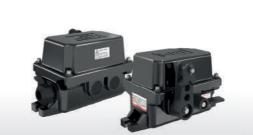
NSR22-PR-EX is used in explosive environment. The products are mounted on the belt with the steel rope pulled parallel to the conveyor belt. The operator provides stop or alarm action by pulling the rope at any point.Optional signal lamp and alarm warning can be
