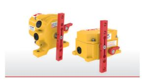
NSR66-PR Series is mounted on the belt with a rope pulled parallel to the conveyor belt. At any point, when the operator pulls the rope, the system can be stopped or an alarm is provided.
